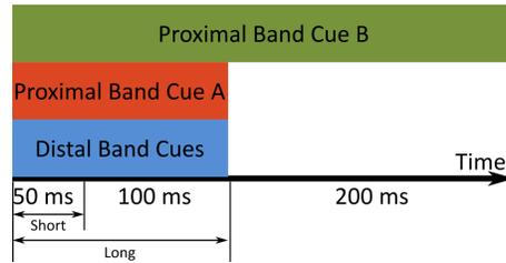
**Fig. 2.** Relative timing of the three haptic cues within a single presentation. The total duration of the haptic presentation is 350 ms. All three cues begin at the same time but have different durations. The Proximal Band Cue B actuates for 350 ms, the Proximal Band Cue A actuates for 150 ms, and a single Distal Band vibrotactor actuates for either 50 ms (short cue) or 150 ms (long cue).
