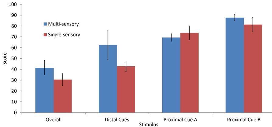
**Fig. 4.** The mean percent correct for both systems is compared ( $N = 8$ ). The overall scores are significantly different ( $p < .01$ ), and the Distal Band vibrotactor accuracies are significantly different ( $p < .01$ ). Error bars denote the 95% confidence interval.
