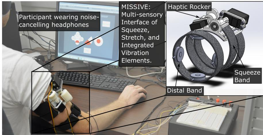
**Fig. 1.** The participant wears the MISSIVE on their upper arm. The bands are spaced three inches center-to-center. The Proximal Band comprises the lateral skin stretch and radial squeeze devices, and the Distal Band houses an array of four vibrotactors spaced  $90^\circ$  apart around the arm.
